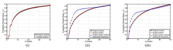
Fig. 2. Distribution of end-to-end packet delays under (i) log-normal shadowing, (ii) Ricean fading, and (iii) Rayleigh fading. (Space-downscaling only.)
