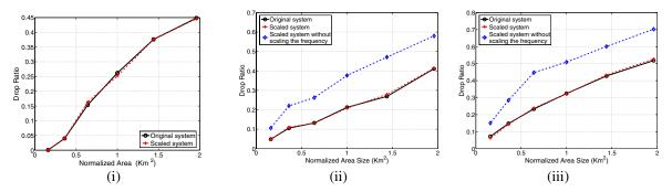
Fig. 3. Packet drop ratio under (i) log-normal shadowing, (ii) Ricean fading, and (iii) Rayleigh fading. (Space-downscaling only.)
