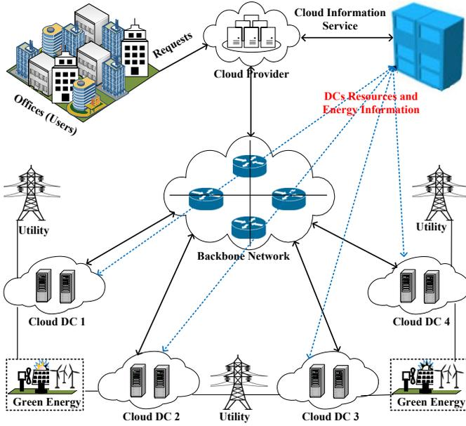
Fig. 1: Architecture of geographically distributed cloud data centers connecting a single cloud provider, several clients, and various energy supplying resources
